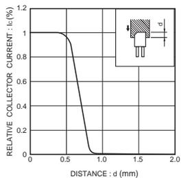
Fig.1 Relative output current vs. distance (I)
